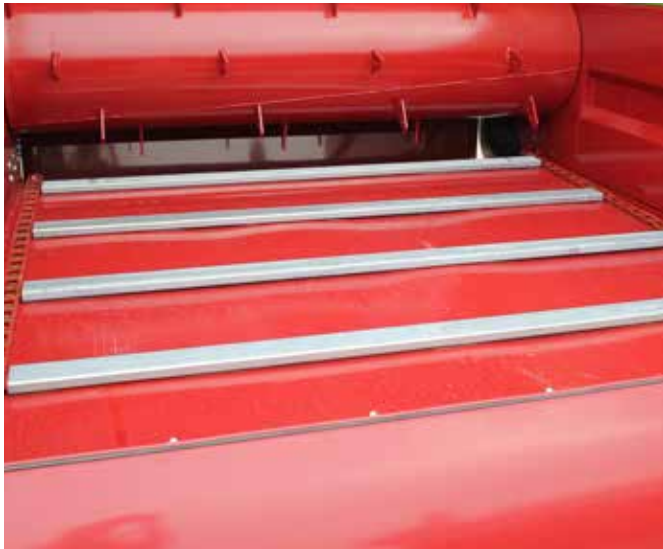
Transport floor The transport floor is fitted with wide, hot-dip galva-nised transport bars. The speed can be continuously adjusted from the tractor via a Bowden cable.
