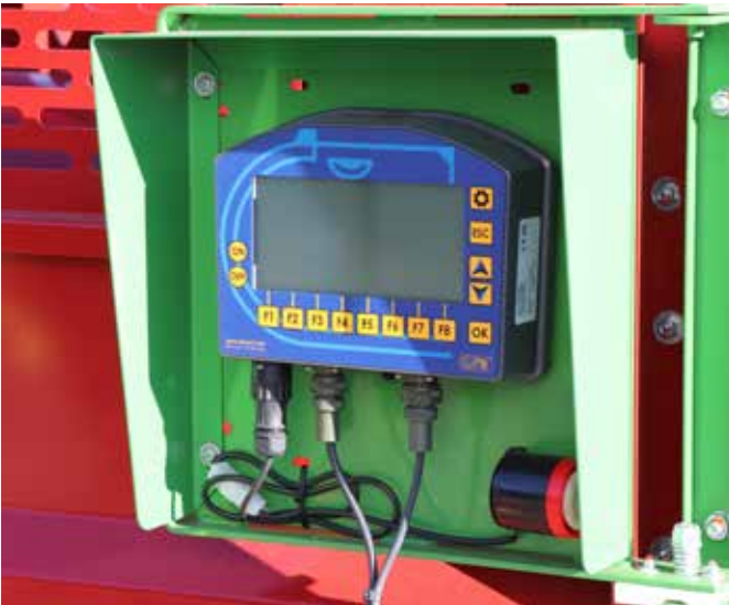
Optional weighing device Block distribution trolleys can be fitted with an opti-onal weighing system, e.g. the PTM HL 50 model. This allows for the management of up to 50 recipes, each with up to 30 components.
