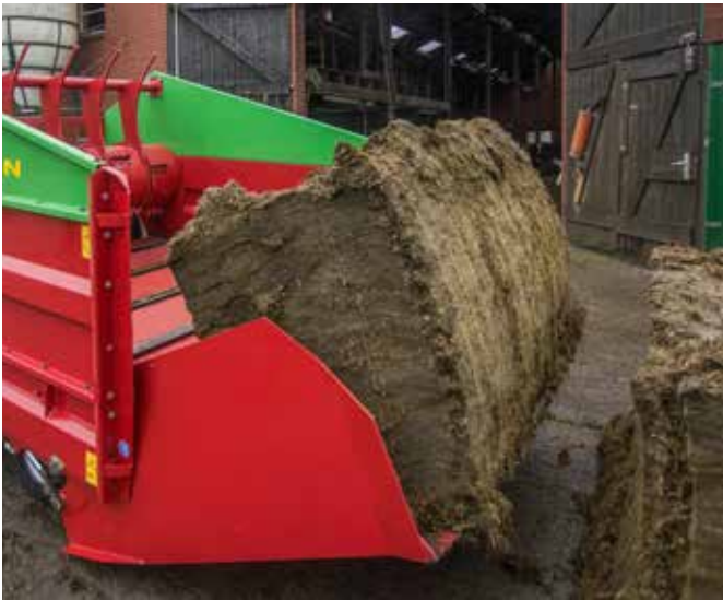
Hydraulic loading door Silage blocks are simply tipped onto the conveyor belt using the loading shovel. The loading shovel can also be used to pick up bulk materials.
