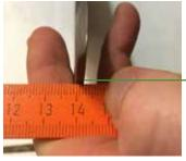
Knife tip 3 mm of residual thickness
