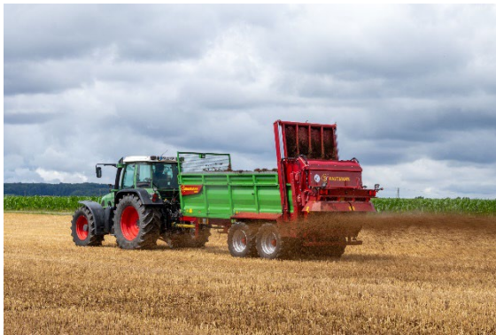
Figure 2: Foldable attachments and universal spreader with cardan drive for versatile use
