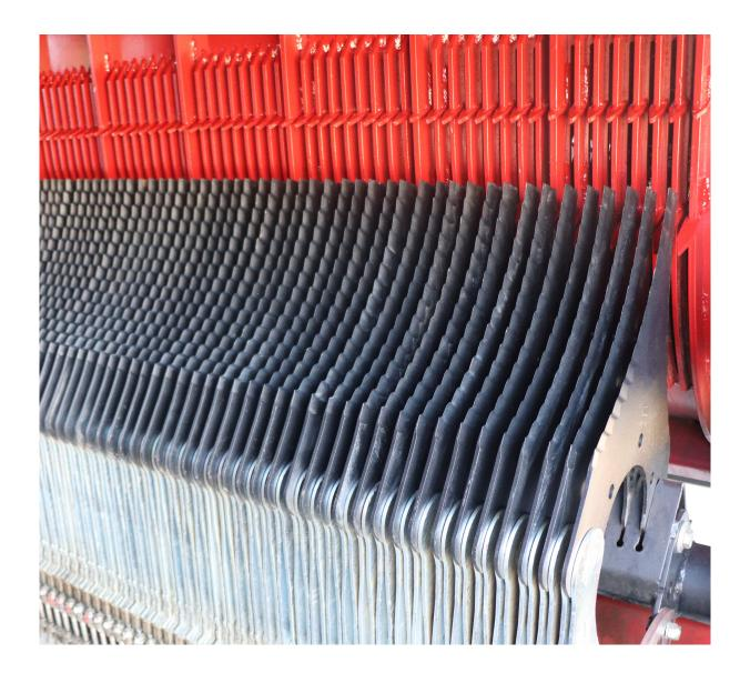
Magnon 11 (2): The cutting unit of the Magnon 11 is equipped with 84 turnable knives.
