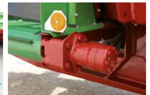
Hydraulic motors – depending on the application, you can select from a range of motors of different speeds.
